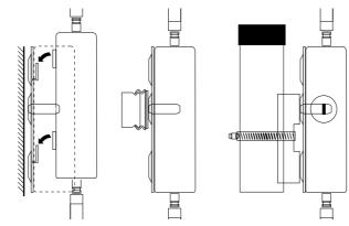
Snap the housing of the device with the four rear openings into the tabs of the base plate.
